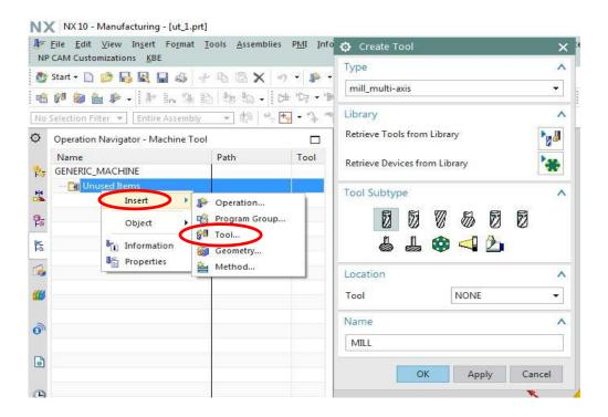
In the <<Tool>> Tab you define geometry, dimensions and cut angles of the cutter
